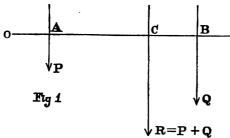
Through O draw a perpendicular to the lines of action
